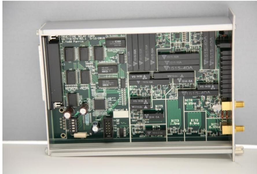
A photograph of a phasing card from one of the new MSI radars is shown in Figure 5. One of these cards is
